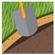
**STEP 1:** Using a hose or rope, make a guide for your edging to follow. If the ground is relatively soft you are good to go. If not, you may need to loosen the ground with a flat spade or pickaxe to ensure the edging can be installed with difficulty.
